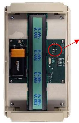
Eight individual stopwatches (A to H) each can be operated by it's individual switch:
